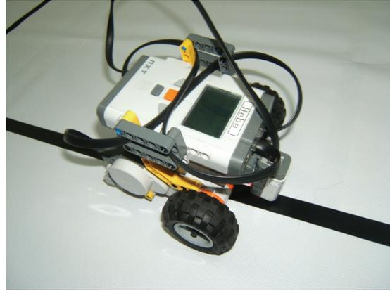
Fig. 5 The experimental Lego-NXT mobile robot
