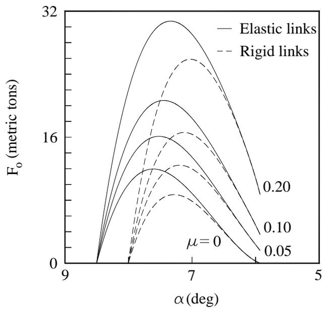
Fig. 7 Thrust applied to the crosshead versus angle  $\alpha$  for showing the two effects.
