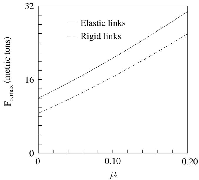
Fig. 8. Maximum thrust applied to the crosshead versus the friction coefficient.
