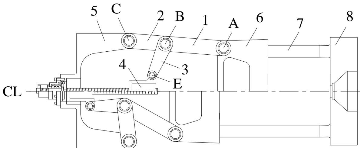
Fig. 1. Four-point double-toggle mold-clamping mechanism.
