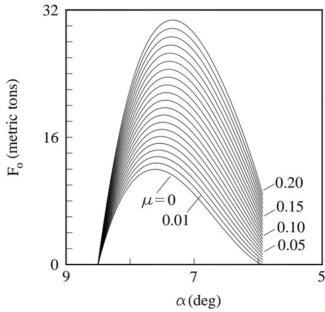
Fig. 6. Thrust applied to the crosshead versus angle  $\alpha$  for several frictional coefficients.
