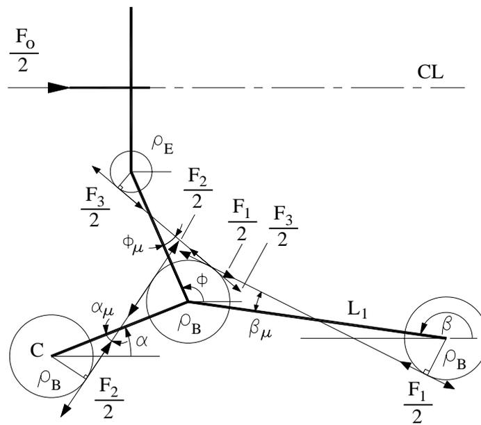
Fig. 3. Toggle linkage subjected to loading during the real mold clamping process.
