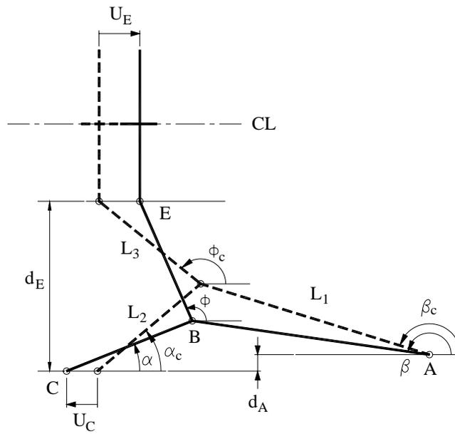
Fig. 2. Geometry of the toggle linkage during real mold clamping.
