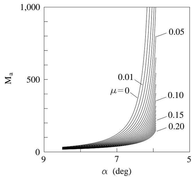
Fig. 5. Mechanical advantage versus angle  $\alpha$ .
