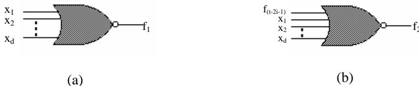
Fig. 5(a) Output gate of original NOR network; (b) Output gate of new network
