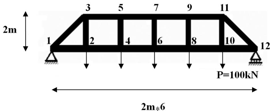
Figure 8. Structure of plane frame bridge
