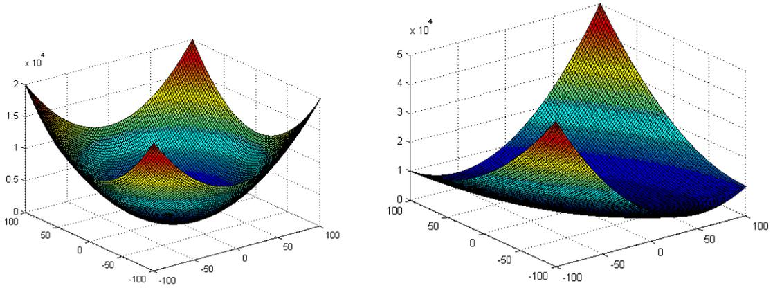
(a)  $F_1(X)$  Spherical (b)  $F_2(X)$  Quadric
