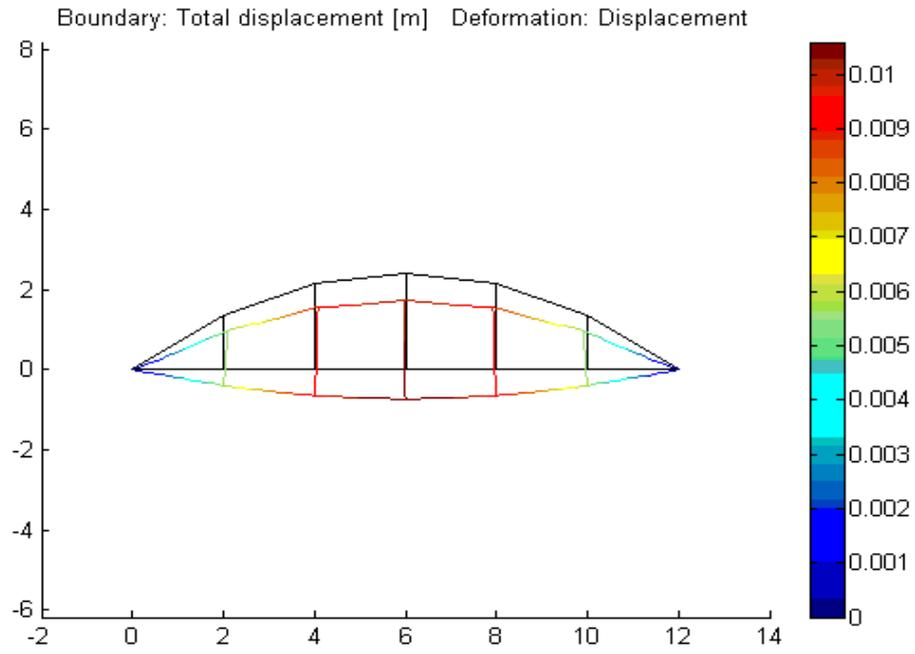
Figure 10. The deformation of the optimum design of plane frame bridges
